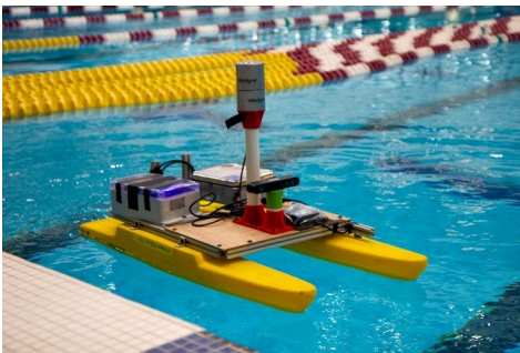
Fig. 9: Indoor testing of our small scale model vessel, Athena , on the water at the MIT Zesiger Athletic Center pool.
