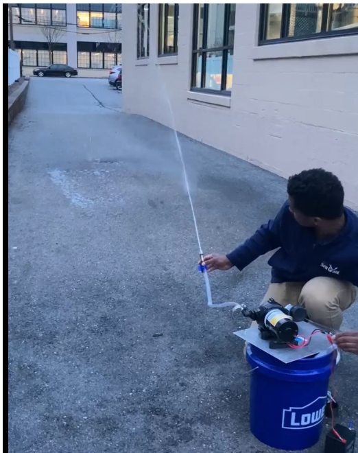
Fig. 11: Experimental water gun mechanism set up at MIT Sea Grant to determine trajectory of the water output.
